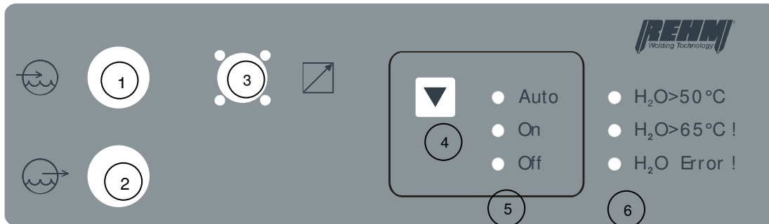
Figure 5: Operating panel for TIG – COOL CART 2000 / TIG – COOL 2000
